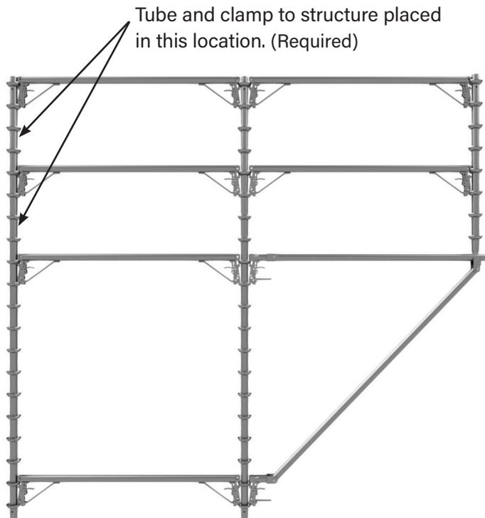
Attach scaffold to a permanent structure capable of preventing tipping of the scaffold.
