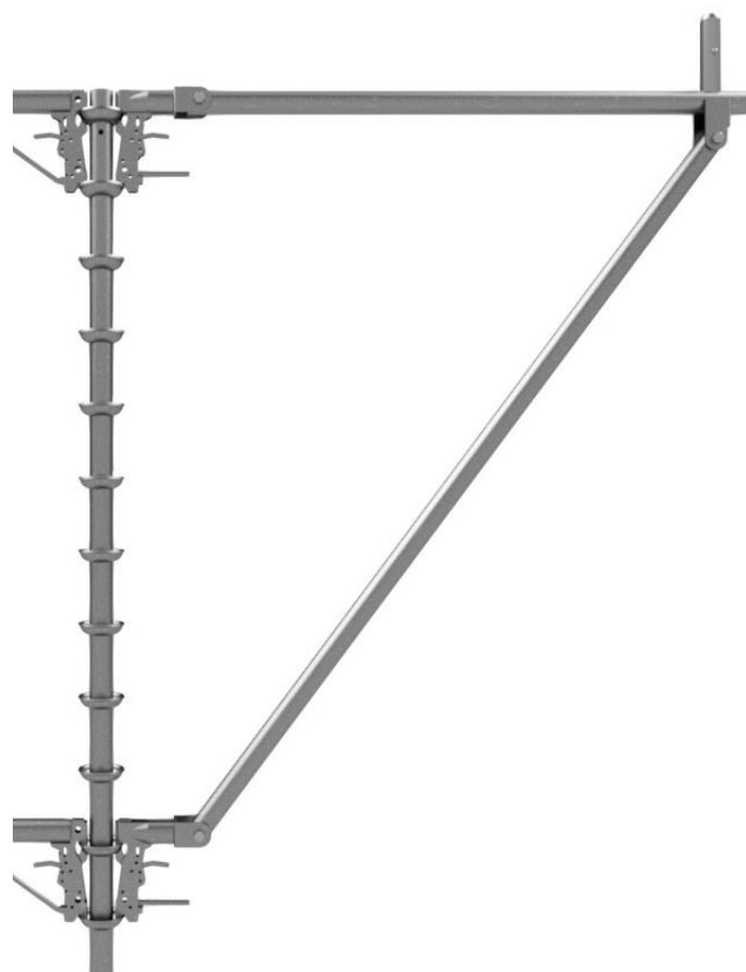
Excel folding side brackets are designed to provide scaffold deck extensions out to six (6) feet. They are also designed to fold up, so that they can be used inside vessels or places with narrow access where a normal side bracket will not fit.
